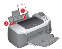
Make sure that Basic Mode is selected (the Basic Mode light is flashing).
